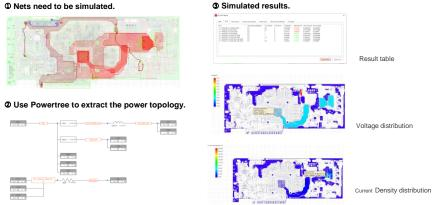
Notus is a simulation platform for signal integrity, power integrity and thermal analysis of chip, package and board. Notus uses a variety of electromagnetic technologies to provide complete simulation process of different applications.
